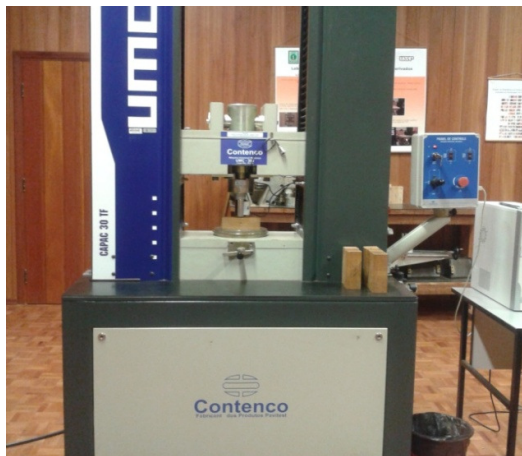
Figure 1 - Machine used in the Janka hardness testing
